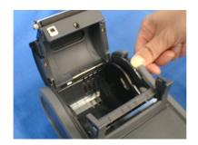
2. When using the label continuous issuing mode: Fold the peeler holder under the peeler cover. This covers the label peeler detector.
